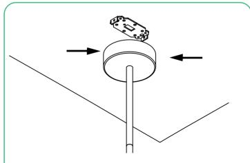
Screw canopy of light fitting over bracket, using the two screws provided.
