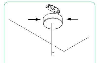
Screw canopy of light fitting over bracket, using the two screws provided.
