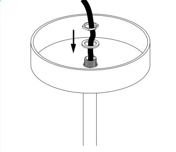
Screw rod into canopy using nut and washer.
