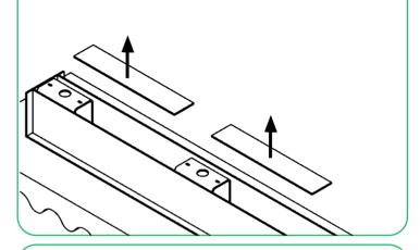
Locate wiring terminal, which connects to driver near the centre of LED base.
